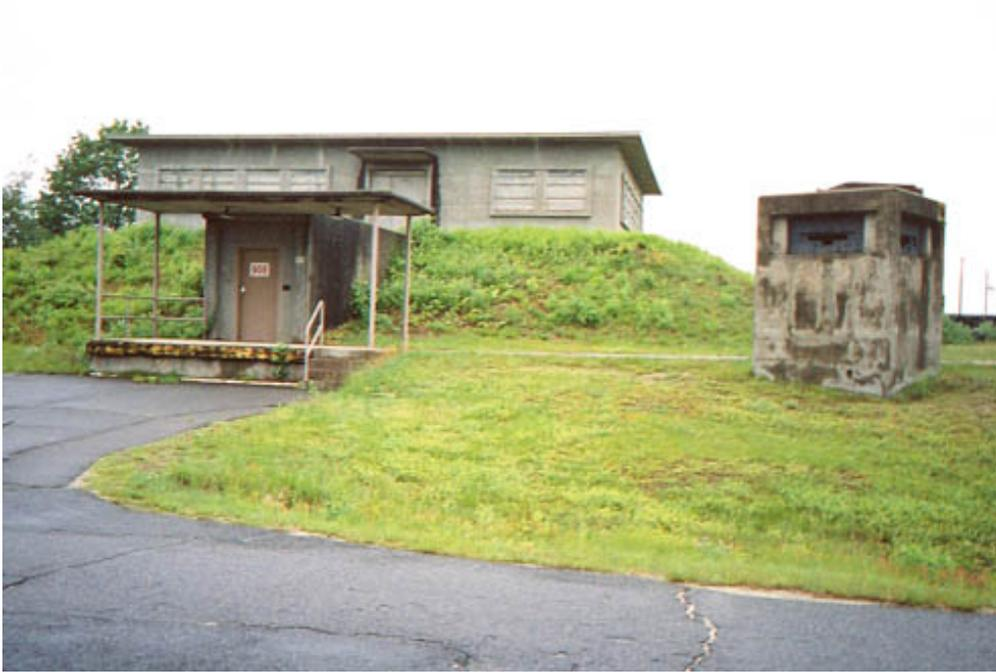
The newer Building 908 where nuclear capsules were stored. The upper structure was a fake building made of solid concrete. The lower entrance led to a vault door that accessed a corridor with 2 doors on either side. These were bank-type vault doors, not blast doors.
